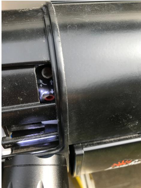
We learned that to adjust the in/out travel of the awning the adjustment screws are in the rear cap of the case. These will adjust the travel of the awning. Just turn a little bit, like maybe 1/4 turn to see what is happening. It turned out that our's didn't need adjusting, but it's good to know for future reference.
