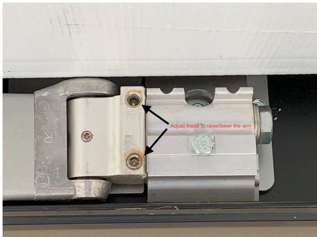
We then learned that each arm has adjustment screws to provide better fit to the awning case. By turning these adjustment screws ( 4mm allen wrench) we were able to raise the knuckle part of the right arm to provide a smooth operation. Now the awning doesn't hang up at all and closes completely.
