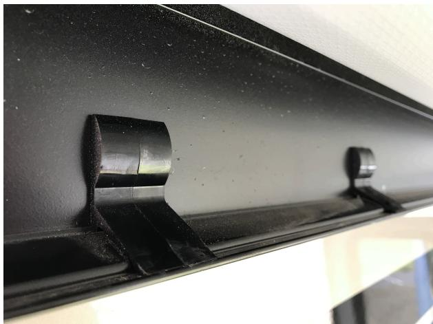
I did notice that our awning came with some ramps installed near the middle inside the case. I presume this was to help the knuckles of the arms to travel over the lip while entering/leaving the case. They are moveable and should be lined up to match the location of the knuckles.
