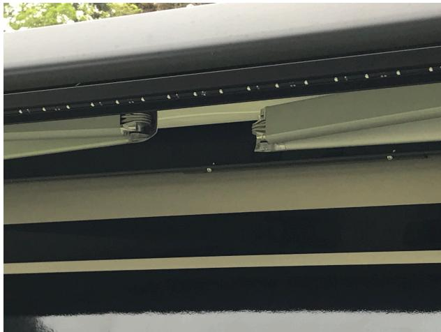
We then noticed that the right (forward) arm was a little lower than the left and was hanging up while extending and retracting. It would keep the awning from closing completely.
