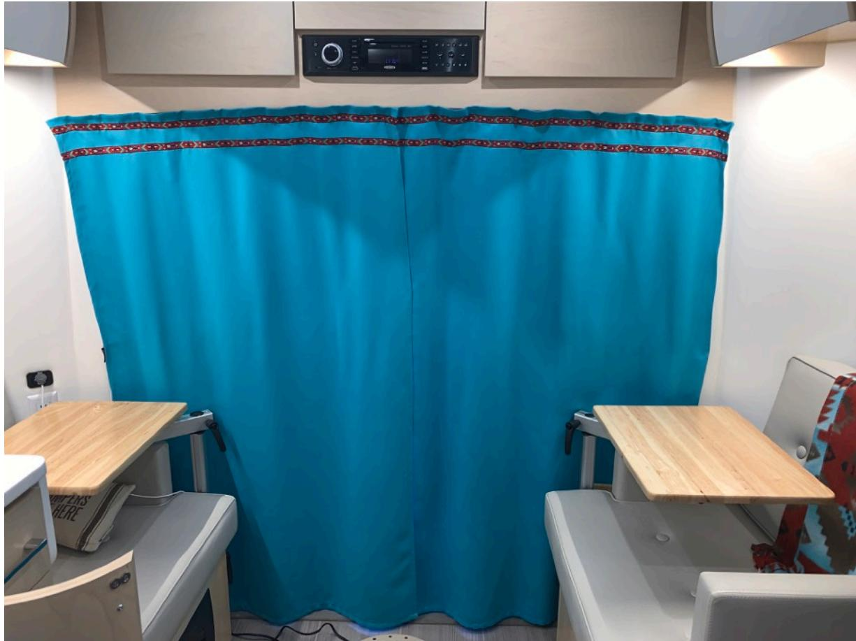
The reason for a curtain between the cab and the living space of our Unity is to help regulate the temperature in the living space. When it's really hot outside, the glass of the cab lets in a lot of heat. A curtain helps restrain it from the living space. Same thing when it's cold; the curtain keeps the cold air from the non-insulated cab from encroaching into our heated living space.
